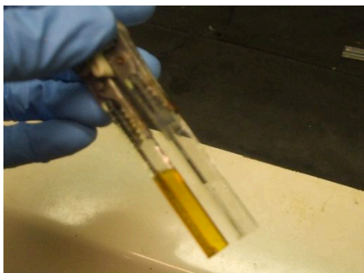
Figure 2: CdSe thin film prepared by EPD
