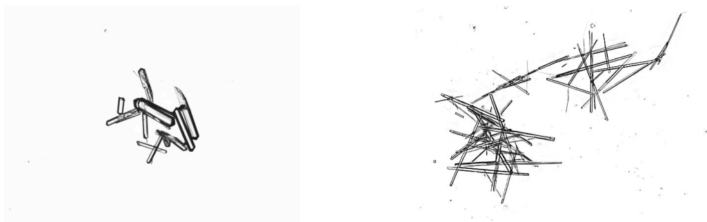
Figure 2: synthetic hydroxyapatite crystals with a 5:3 (left) and 3:5 (right) calcium:phosphorous ratio
